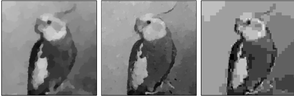
Fig. 10. Reconstruction of Bird (256 × 256) at 1/8 bpp ( M = 8,192 ) using three distinct methods. From left to right: GF using M_0^2 = 256^2 , L = 8 , and \Lambda = 1/64 without (SNR: 21.65 dB, BSNR: 23.4 dB) and with finite differentiation (SNR: 19.79 dB, BSNR: 25.65 dB), and JPEG (SNR: 19.68 dB, BSNR: 22.66 dB). The plain-JPEG compression is performed at its lowest quality settings, which approximately yields the same bitrate (the corresponding file size is 10,280 bits, including header data).
