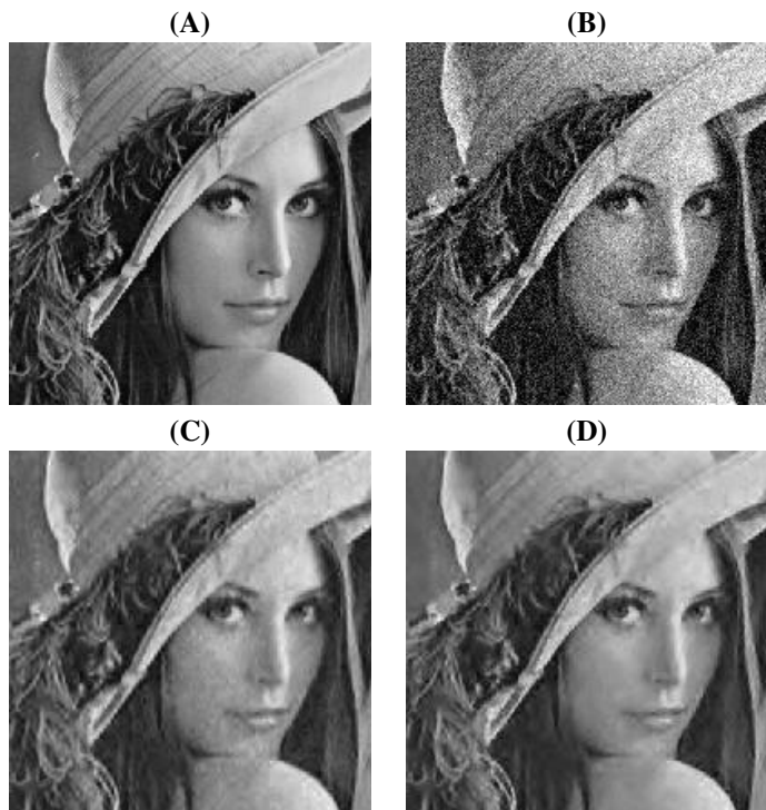
Fig. 6. (A) Part of the noise-free Lena image. (B) Noisy image: PSNR = 20.17 dB. (C) BayesShrink: PSNR = 29.31 dB. (D) Our method: PSNR = 30.36 dB.
