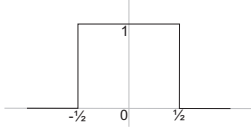
FIGURE 1. The box function (the B-spline basis of degree 0).
