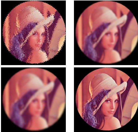
FIGURE 5. The Lena image is rotated repeatedly in 36 steps of 10 degrees each. For every iteration, the outcome of the previous step is interpolated on a rotated grid. Top left: nearest-neighbor interpolation. Top right: linear interpolation. Bottom left: cubic reconstruction without prefilter. Bottom right: prefiltered cubic interpolation.
