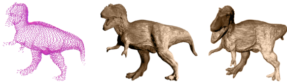
Fig. 7 Interpolation of a parameterized point cloud. The dinosaurs (middle and right) are smooth reconstructions obtained by interpolating the point cloud on the left. Our surface construction is affine invariant and hence, rotating the shape is simply performed by rotating the point cloud.
