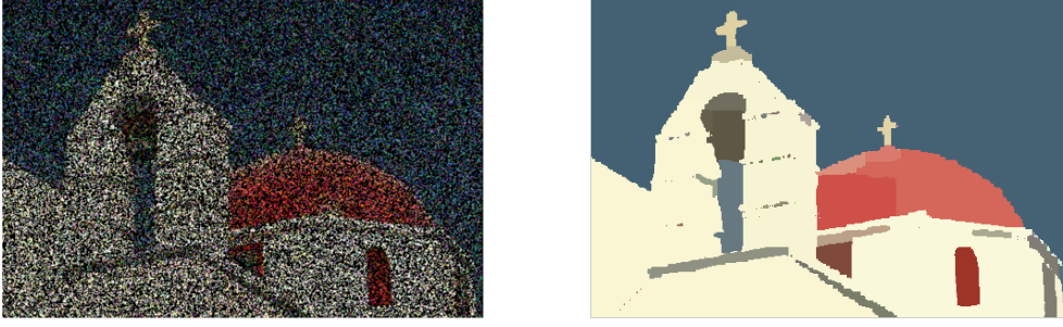
Fig. 3: Left : Image corrupted by Gaussian noise of \sigma = 0.2 ; 60% of the pixels are missing (marked as black); Right : Restoration using our method ( \gamma = 0.3 ).
