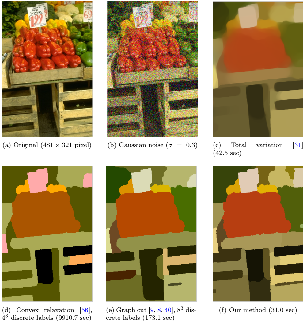
Fig. 5: Comparison of segmentations of a natural image ( \gamma = 2.0 ). Total variation minimization (model parameter \lambda = 4.0 ) tends to smooth out some of the segment boundaries (c). Among the Potts segmentation approaches (d-f), the proposed method is the fastest.
