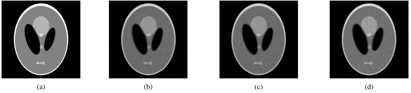
Fig. 3. SPS reconstructions of a SL sinogram with 50 views \times 512 pixels and additional Gaussian noise with \sigma = 2.4\% of the sinogram mean. (a) Phantom. (b) Reconst. with SPS-PSWF. (c) Reconst. with SPS-KB. (d) Reconst. with SPS-BSPLINE.
