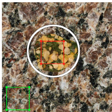
Fig. 4. Extraction of \Omega_C (red ROI) and \Omega_B (green ROI) for training Fisher's LDA. (For interpretation of the references to color in this figure legend, the reader is referred to the web version of this article.)
