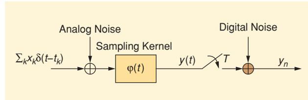
[FIG1] Block diagram representation of the sampling of an FRI signal, with indications of potential noise perturbations in the analog, and in the digital part.
