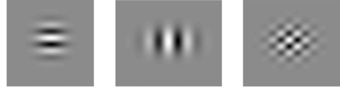
Fig. 4. Wavelets associated with the separable basis. The figure shows the LH, HL, and HH wavelets in the space domain.
