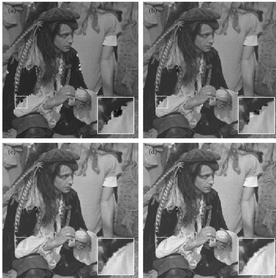
Fig. 4. Phase unwrapping results for Man image of size 256 \times 256 when the amplitude is a = 7 . (a) LS (SNR = 18.14 dB); (b) IRLS (SNR = 24.23 dB); (c) PUMA (SNR = 27.46 dB); (d) IRTV (SNR = 29.22 dB).
