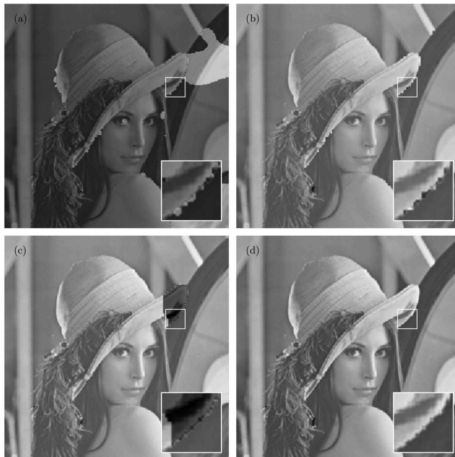
Fig. 3. Phase unwrapping results for Lena image of size 256 \times 256 when the amplitude is a = 9 . (a) LS (SNR = 7.33 dB); (b) IRLS (SNR = 25.50 dB); (c) PUMA (SNR = 15.51 dB); (d) IRTV (SNR = 30.47 dB).
