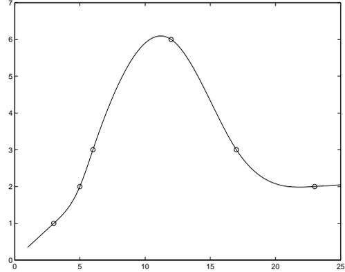
Figure 1: Interpolation from function values.
