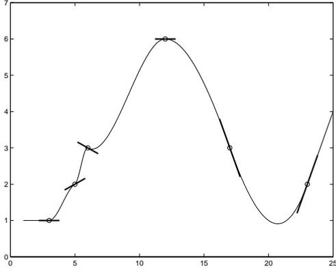
Figure 2: Interpolation from function values and derivatives.
