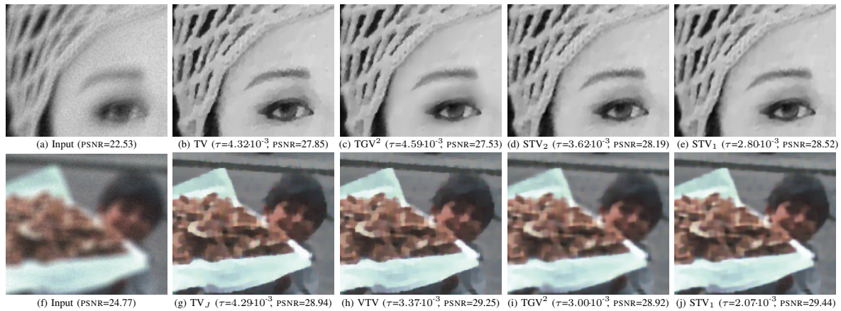
Figure 6. Image deblurring examples: close-ups of inputs and optimum results. Top row: grayscale deblurring of an input with motion blurring and noise level \sigma_w = 0.025 . The ground truth corresponds to the grayscale version of the image in row 3, column 4 of Figure 2. Bottom row: color deblurring of an input with uniform blurring and noise level \sigma_w = 0.025 . The ground truth corresponds to the image in row 3, column 6 of Figure 2. For each result, the individualized regularization parameter \tau and corresponding optimum PSNR are reported.
