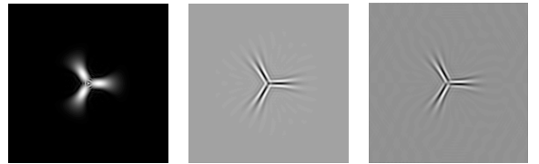
Fig. 1: 3-fold symmetric wavelet in the space domain; from left: magnitude, real and imaginary parts. Harmonics: S = \{3n : n = 0, \dots, 9\} .
