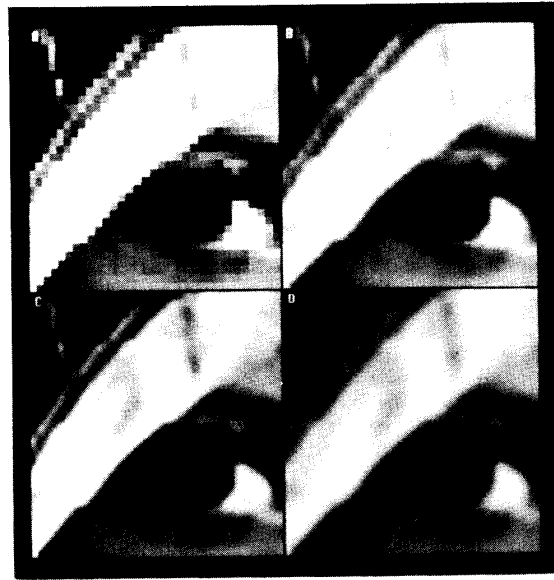
Fig. 6. Comparison of interpolation algorithms for the magnification with a zooming factor 8 of a 32 \times 32 detail of the standard girl image. (a) 0 order interpolation, (b) bilinear interpolation, (c) bicubic spline interpolation, (d) smoothing by indirect bicubic spline transform.
