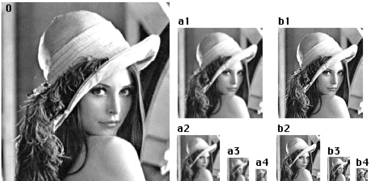
Fig. 8. Comparison of image pyramids. (0): Initial test image (level 0), (a1–b4): levels 1 to 4 of Burt's Gaussian pyramid with a = 3/8 , (b1–b4): levels 1 to 4 of the least squares cubic spline pyramid.
