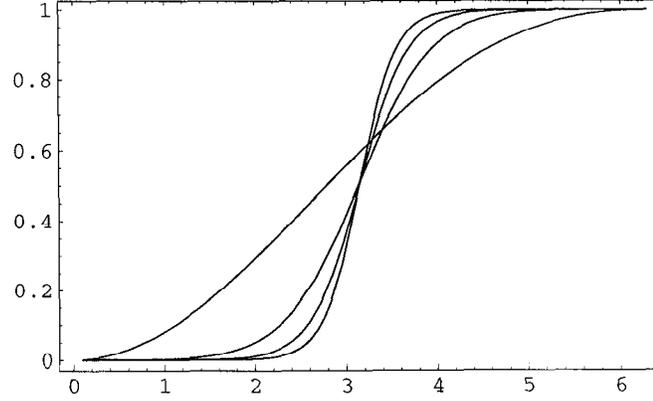
Fig.2. Frequency plot of the error kernels for the orthogonal projection on the spline spaces of degree 0, 1, 2, and 3. The higher order kernels are consistently smaller below the Nyquist frequency  $\omega = \pi$ . This explains why higher order splines provide a better approximation of functions that are predominantly lowpass.
