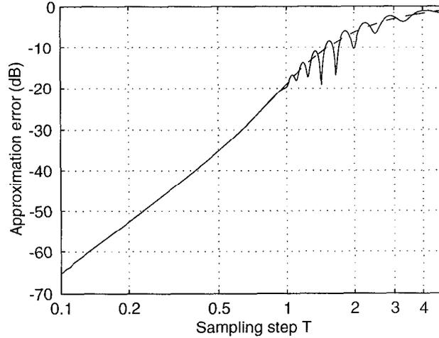
Fig.1. Least squares approximation error of the function  $f(x) = e^{-x^2/2}$  by cubic splines as a function of the sampling step  $T$ . The error estimate  $\mathcal{E}_f^2(T)$  (dashed line) is an unbiased smoothed version of the true error (solid line).
