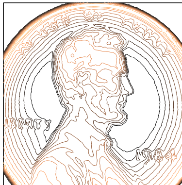
Figure 11.7. The depth of a mold used to mint the U. S. one cent coin.
