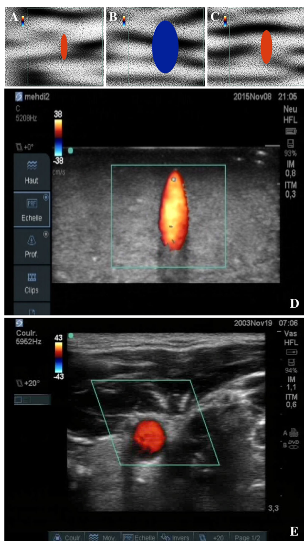
Fig. 4 A comparison of example synthetic test images for angle (a), speed (b), area detection (c), phantom images (d), and natural images (e). The green quadrangle surrounding the vessel and the colorscale displayed by our ultrasound machine were reproduced on synthetic images to enable correct analysis
