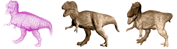
Figure 4: Interpolation of a parameterized point cloud. The dinosaurs (middle and right) are smooth reconstructions obtained by interpolating the point cloud on the left. Our surface construction is affine-invariant, which implies that a rotation of a shape is simply obtained by rotating the point cloud.
