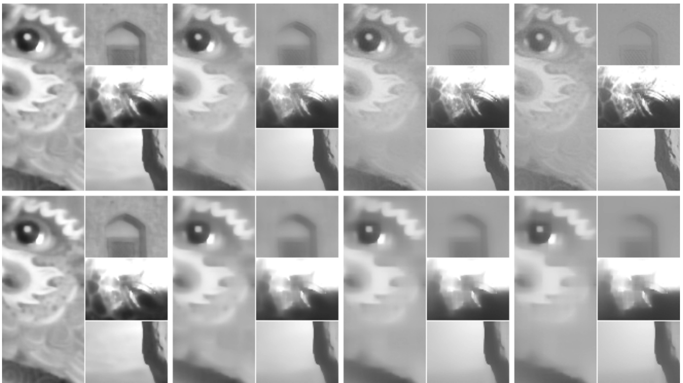
Fig. 10. Application of the bilateral filter (top row) and the BEEPS (bottom row) to the cutouts from Figure 8. The bi-exponential spatial filter takes the contra-decay \lambda \in \{0.5, 0.8, 0.9, 0.95\} , from left to right. The standard deviation of the Gaussian range filter is kept constant, with \sigma = 50 .
