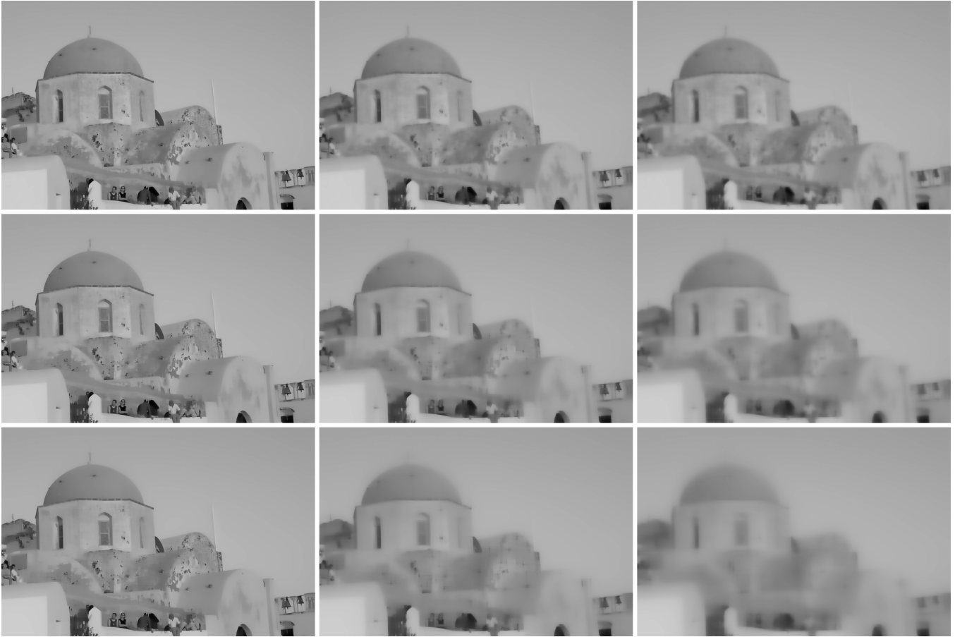
Fig. 4. Gallery of results of the BEEPS applied to the GreekDome image. The spatial smoothing increases from top to bottom with \lambda \in \{0.8, 0.9, 0.95\} . From left to right, there is an increase in the standard deviation of the range filter \sigma \in \{20, 50, 100\} . The original image is visually close to the topmost, leftmost image in the gallery. The computational cost was identical for all images.
