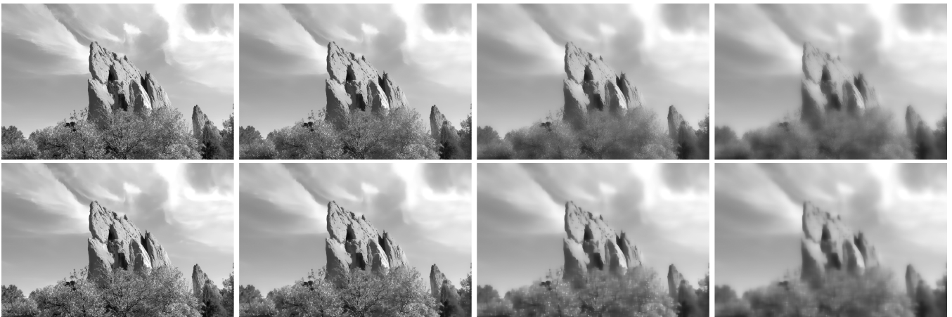
Fig. 5. Bilateral filter (top row) and BEEPS (bottom row), as applied to the Rock image. The contra-decay is constant with \lambda = 0.9 . The standard deviation of the range filter increases from left to right with \sigma \in \{10, 20, 50, 100\} .
