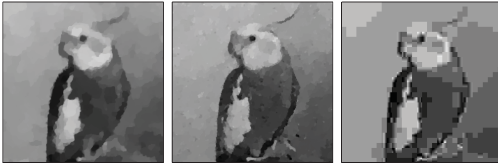
Fig. 9. Reconstruction of Bird (256 × 256) at 1/8 bpp ( M = 8 \cdot 192 ) using three distinct methods. From left to right: GF using M_0^2 = 256^2 , L = 8 , and \Lambda = 1/64 without (SNR: 21.65 dB and BSNR: 23.4 dB) and with finite differentiation (SNR: 19.79 dB and BSNR: 25.65 dB), and JPEG (SNR: 19.68 dB and BSNR: 22.66 dB). The plain-JPEG compression is performed at its lowest quality settings, which approximately yields the same bit rate (the corresponding file size is 10 280 b, including header data).
