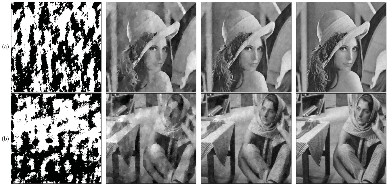
Fig. 6. Results on Lena and Barbara ( 512 \times 512 ) for distinct numbers L of acquisitions using M_0^2 = 512^2 and \Lambda = 1 without finite differentiation ( M = L \cdot 512^2 measurements in total). (a) First acquisition \gamma_1 of Lena using our model, and reconstruction from one ( M = 262\,144 , SNR: 17.49 dB, and BSNR: 22.35 dB), two ( M = 524\,288 , SNR: 22.42 dB, and BSNR: 24.61 dB), and four ( M = 1\,048\,576 , SNR: 26.46 dB, and BSNR: 27.13 dB) acquisitions. (b) First acquisition \gamma_1 of Barbara using our model, and reconstruction from one ( M = 262\,144 , SNR: 13.96 dB, and BSNR: 16.09 dB), two ( M = 524\,288 , SNR: 17.69 dB, and BSNR: 17.74 dB), and four ( M = 1\,048\,576 , SNR: 20.3 dB, and BSNR: 20.28 dB) acquisitions.
