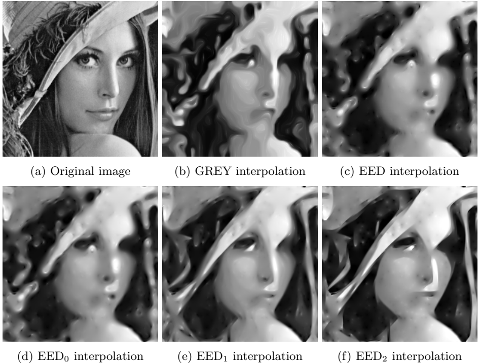
Figure 2.5: Ideal interpolation of Lena ( 256 \times 256 crop) from 2% of samples.
