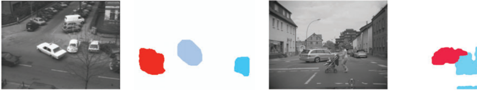
FIG. 7. Result for two traffic scenes. From left to right: image of the taxi scene (source: http://i21www.ira.uka.de/image_sequences/ . Last accessed December 12, 2014), partitioned optical flow by the direct algorithm ( \lambda = 6 ) using frames 10 and 17, first image of the stroller scene (source: http://ccv.wordpress.fos.auckland.ac.nz/eisats/ . Last accessed December 12, 2014 [7]), partitioned optical flow by the direct algorithm ( \lambda = 2.5 ).
