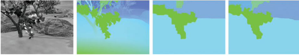
FIG. 6. Result for the images ‘Grove2’. Left to right: first test image, ground truth, partitioned flow with non-isotropic and isotropic discretization ( \lambda = 0.6 ) (source: http://vision.middlebury.edu/flow/ . Last accessed December 12, 2014 [6]).
