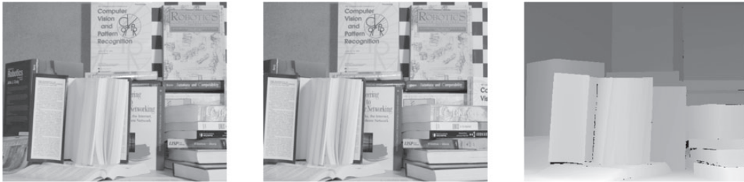
FIG. 1. Left and middle: Two images taken by a stereo camera. The shift between the images is clearly visible. Right: True disparity encoded by different gray values which shows the depth of the different objects in the scene (source: http://vision.middlebury.edu/stereo/ . Last accessed December 12, 2014).
