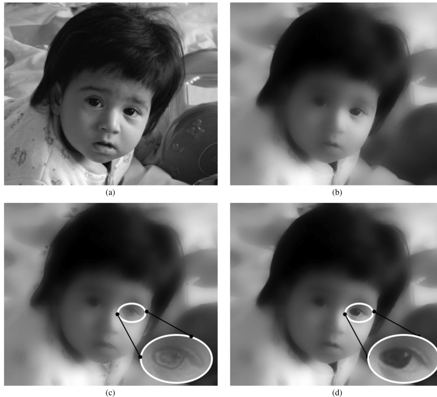
Fig. 3. Comparison of various implementations of the Gaussian bilateral filter on the grayscale image Isha of size 600 \times 512 . The filter settings are \sigma_s = 15 and \sigma_r = 80 . (a) Original image. (b) Direct implementation of the bilateral filter. (c) Output obtained using polynomial kernel [2]. (d) Output of our algorithm. Note the strange artifacts in (c), particularly around the right eye (see zoomed insets). This is on account of the distortion caused by the polynomial approximation shown in Fig. 2. The standard deviation of the error between (b) and (c) is 6.5, whereas that between (b) and (d) is 1.2.
