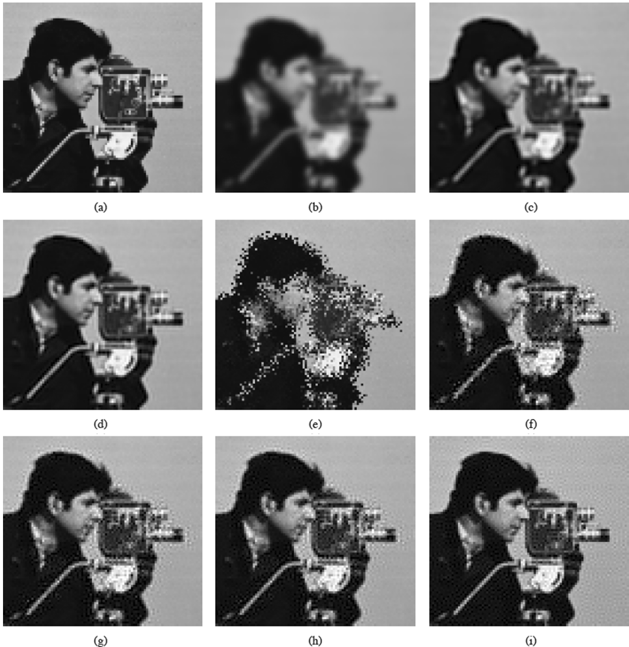
Fig. 7. Images obtained after nine rotations of angle 2\pi/9 on a part of the camera image depicted in (a), using (b) bilinear, (c) bicubic, and (d) O-MOMS interpolation, and our method in three shears with filters (e) h_\tau^0 (nearest neighbor), (f) h_\tau^{1,1} , (g) h_\tau^{1,2} , (h) h_\tau^{1,3} , (i) h_\tau^\infty (sinc). The PSNRs are from (b) to (i): 21.19, 25.15, 29.77, 15.63, 23.07, 25.05, 26.02, and 28.67 dB, respectively. The images obtained with h_\tau^{2,2} , h_\tau^{2,3} , and h_\tau^{2,4} , not reproduced here, give PSNRs of 26.07, 27.24, and 27.93 dB, respectively.
