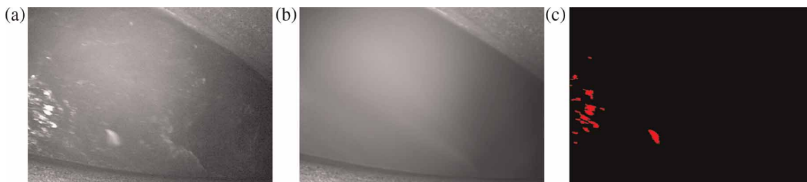
Figure 2 | Image analysis for particle detection. (a) Original infrared image; (b) background estimation; (c) binary image with possible particles for velocity measurement.
