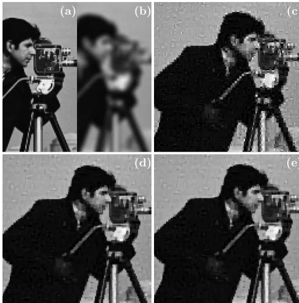
Figure 3.2: Reconstruction of Cameraman from blurry and noisy measurements. (a) original, (b) blurry, (c) standard wavelet-based ISTA (SNR = 19.10 dB), (d) reconstruction with TV (SNR = 21.58 dB), (e) wavelet-based reconstruction with cycle spinning (SNR = 21.58 dB).
