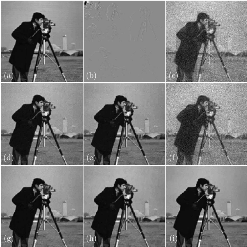
Figure 6.6: Compressive sensing reconstruction of 128 \times 128 Cameraman for a measurement ratio of M/N = 0.7 . (a) original, (b) wavelet decomposition, (c) ortho- l_2 : 10.00 dB, (d) ortho- l_1 : 21.77 dB, (e) ortho-GAMP: 22.54 dB, (f) CS- l_2 : 10.12 dB, (g) CS- l_1 : 24.25 dB, (h) TV: 25.20 dB, (i) CS-GAMP: 26.62 dB.
