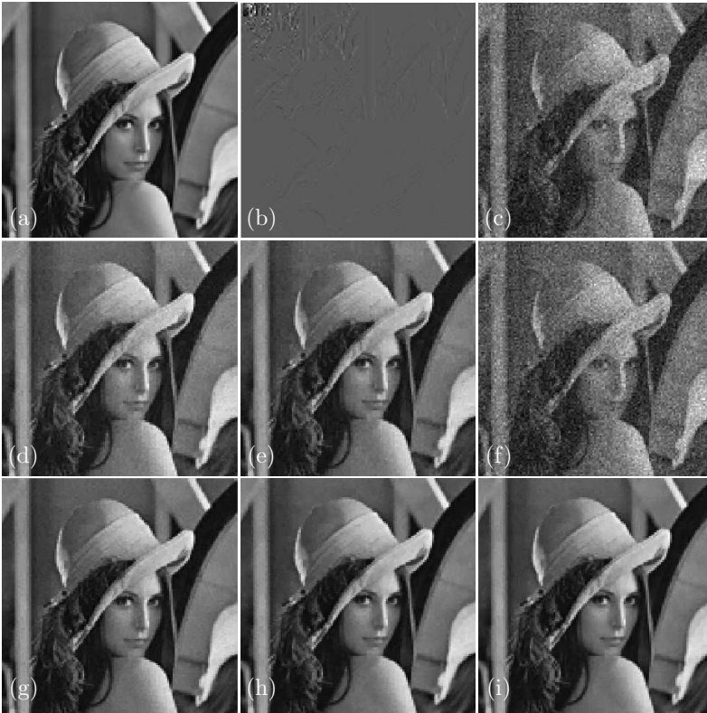
Figure 6.5: Compressive sensing reconstruction of 128 \times 128 Lena for a measurement ratio of M/N = 0.7 . (a) original, (b) wavelet decomposition, (c) ortho- l_2 : 7.71 dB, (d) ortho- l_1 : 17.81 dB, (e) ortho-GAMP: 19.41 dB, (f) CS- l_2 : 7.80 dB, (g) CS- l_1 : 21.02 dB, (h) TV: 22.46 dB, (i) CS-GAMP: 23.52 dB.
