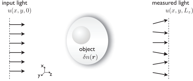
Fig. 1. Visual representation of the scattering scenario considered in this paper. A sample with a real refractive index contrast \delta n(\mathbf{r}) is illuminated with an input light u(x, y, z = 0) , which propagates through the sample, and results in the light u(x, y, z = L_z) at the camera plane. The light at the camera plane is holographically captured and the algorithm proposed here is used for estimating the refractive index contrast \delta n(\mathbf{r}) .
