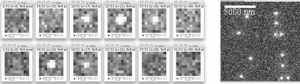
Fig. 2. An example of calibration z-stack data. Shown here on the left are slices of two z-stacks that include a single point-source fluorophores. This fluorophore is captured by two planes which are 1,000[nm] apart along the optical axis in object domain. As the focal plane of the microscope moves away from the objective lens, the maximum response of the fluorophore appears at different slice indices. Our z-stack data simulator chooses random 3D positions for the fluorophores and computes the biplane acquisition images. Misalignment between the two planes is associated with 2D rotation, scaling and defocus. We also include Poisson-type photon emission and additive Gaussian noise models. Maximum projection of a typical calibration z-stack data is shown on the right.
