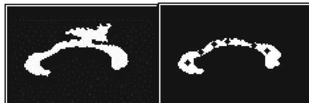
Fig. 14 Result of the border path pruning. The holes are just displayed to show where the centers of the circles are located. In the final images, there will be no holes.
