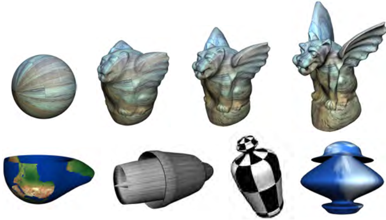
Figure 7.1: Smooth modeling of shapes with spherical topology. A continuous deformation of the sphere into the Gargoyle is shown in the top row, where a wood texture has been added to the surface. The shapes in the bottom row consist of a single surface patch and are constructed through interactive deformation of the sphere. The interpolating structure of the model allows us to intuitively design surfaces that can adopt shapes beyond the classical spherical topology. Our framework is inherently smooth, which facilitates natural texturing.
