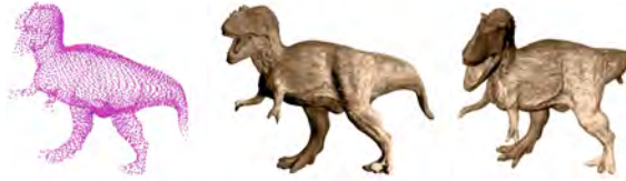
Figure 7.7: Interpolation of a parameterized point cloud. The dinosaurs (middle and right) are smooth reconstructions obtained by interpolating the point cloud on the left. Our surface construction is affine invariant and hence, rotating the shape is simply obtained by rotating the point cloud.
