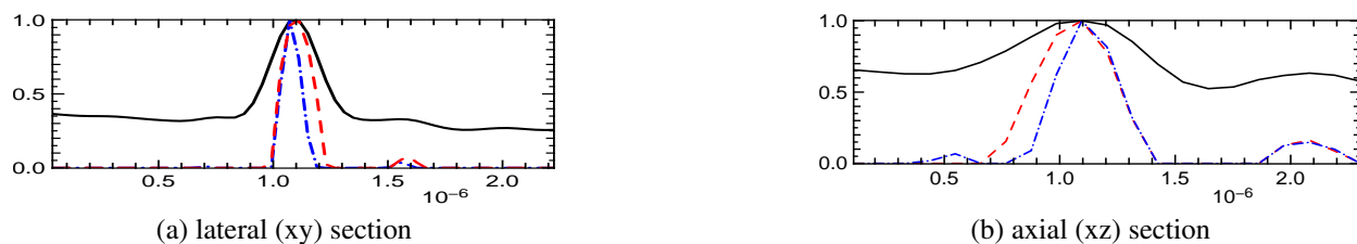
Fig. 2. Lateral and axial profile of the microtubule indicated by the green line on Figure 1.a for the wide field data (solid line), its blind deconvolution (dashed red), and the SIM (mixed blue).
