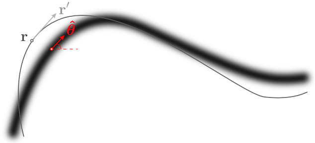
Fig. 2. Schematic representation of the Hermite snake \mathbf{r} , of its derivative in a point \mathbf{r}' , and of its interaction with an object consisting of a dark ridge. The unit vector \hat{\theta} is the best response of the steerable filter for ridge detection. Since an estimation of \hat{\theta} is available for every point of the image, the inner product featured in the snake energy therefore favors tangents aligned to the orientation of best response.
