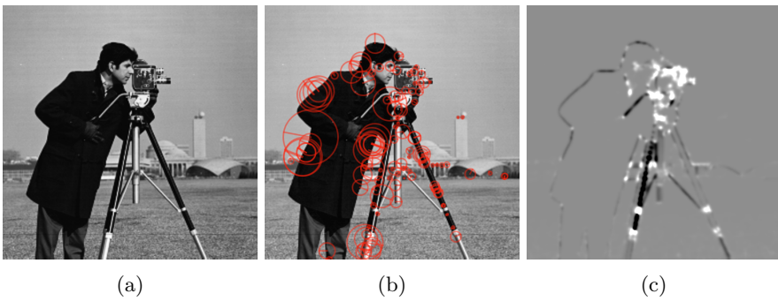
Figure 2.1: Illustration of different approaches for identifying salient points. (a) Input image. (b) Output of a detector providing a set of distinctive points (SIFT). It consists in a discrete list of points locations, scale and main orientation. Here, they are overlaid as circles on the input image, with the circle size depicting the scale and a radius inside it depicting the main orientation. One notices that keypoints are unspecific, e.g. , they are found both on corners and edges. (c) Output of a detector providing a set of points with common properties (Harris corner detector). It yields a magnitude map, which contains at each location on the image an measure of how much the desired feature is present. Here, the brighter an area, the more “corner-like” it is.
