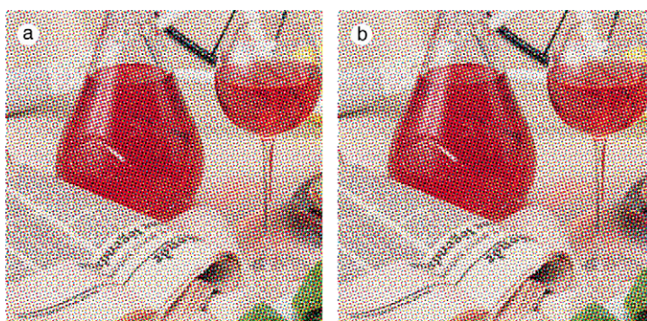
Fig. 7. Normal test image. (a) Halftoned after first-order least-squares prefiltering. (b) Halftoned after second-order least-squares prefiltering.
